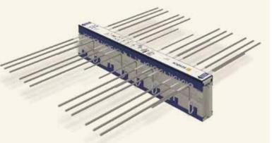
Schöck Isokorb concrete-to-concrete structural thermal break transfers bending moments and shear forces, while preventing heat energy waste, chilled interior floors, and formation of condensation and mould.
