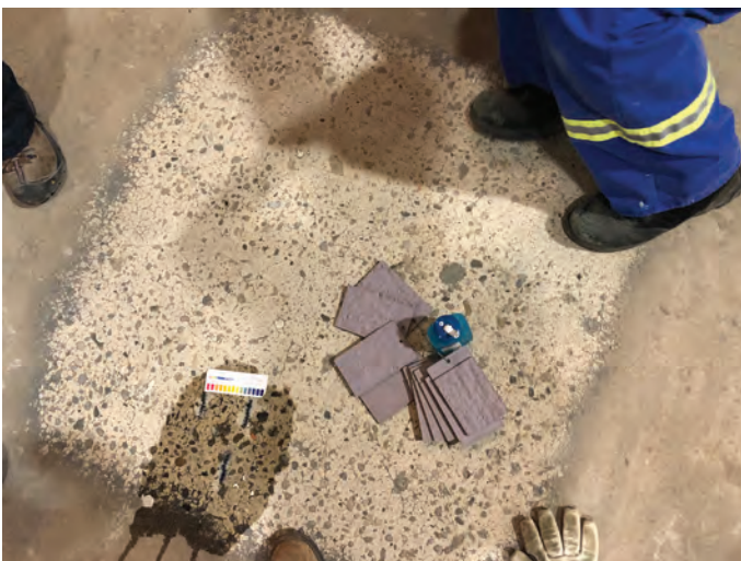
Fig. 5: Determining substrate concrete surface profile (CSP) and pH testing
