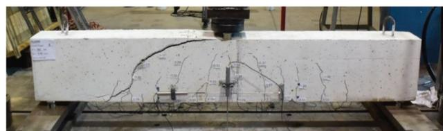
Fig. 12—Traditional size shear specimen: PLS300, load-deformation response and failure behavior.
