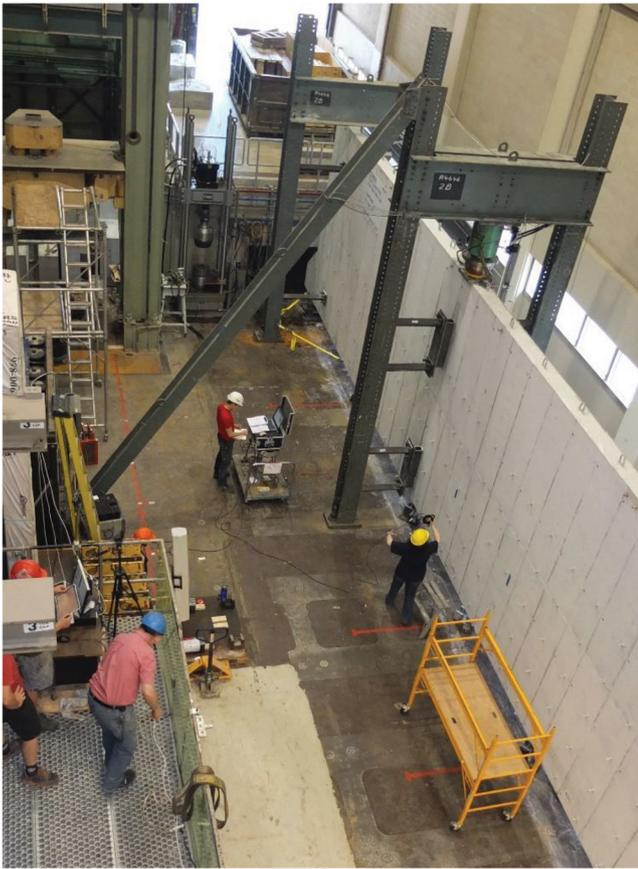
Fig. 3—Loading and lateral bracing of PLS4000.
