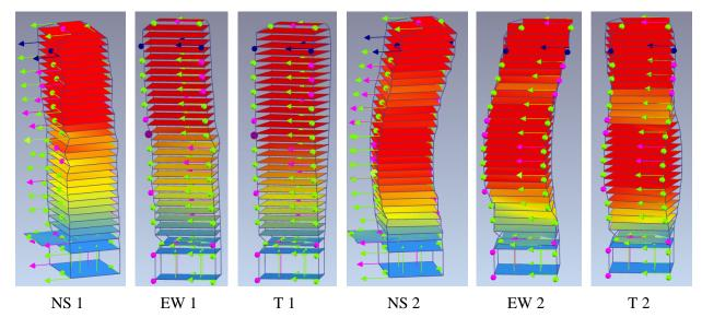
Figure 6: The first six mode shapes from the ambient vibration test.
