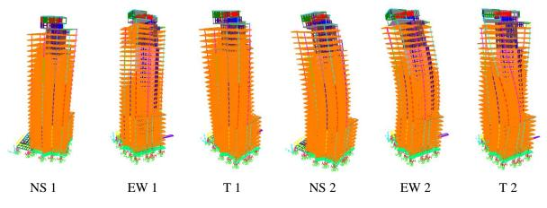
Figure 8: The first six mode shapes from the FE model without the basement
